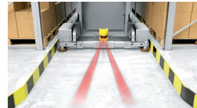
Mobile personal protective equipment with laser scanner
