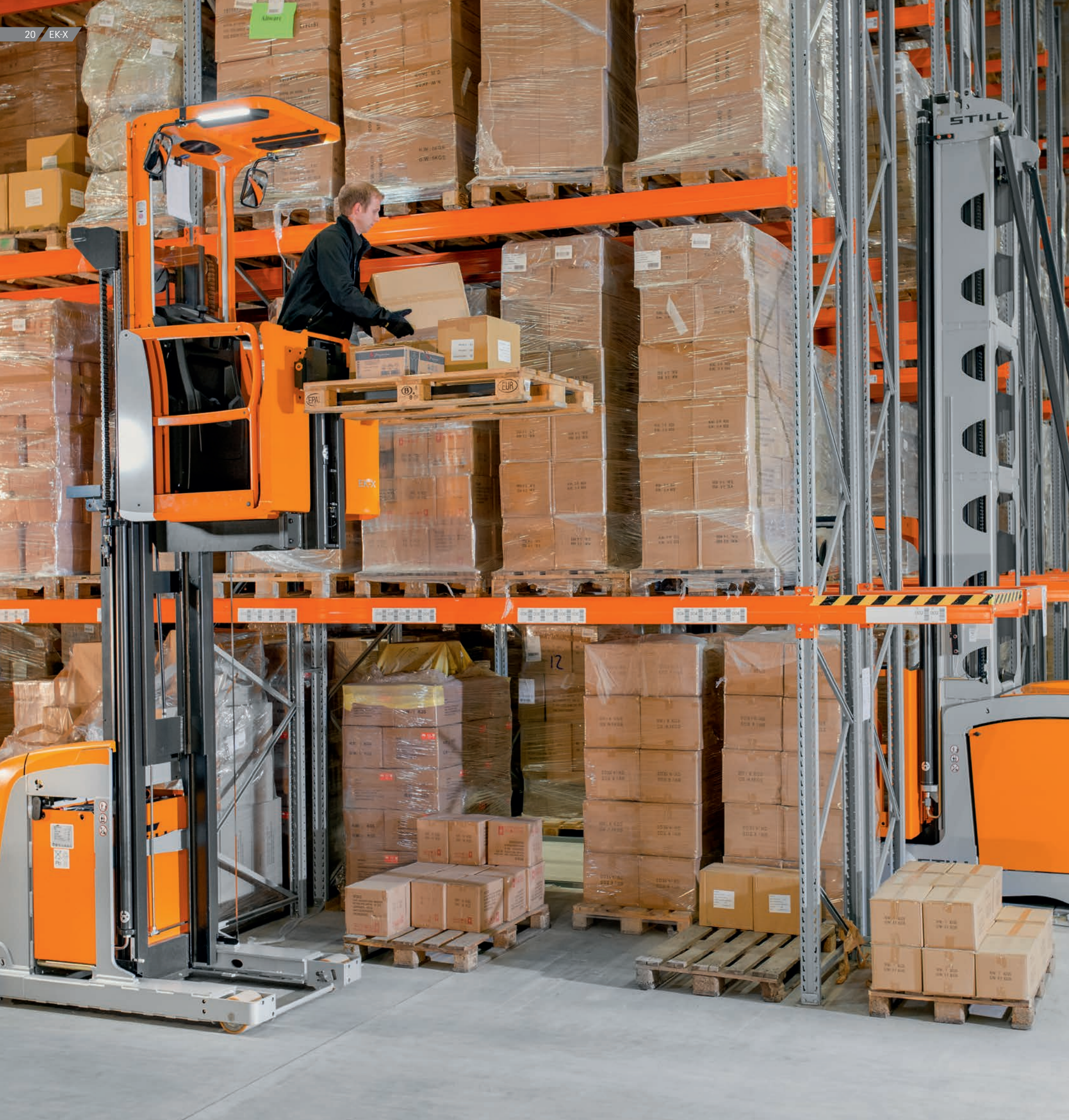
EK-X vertical order picker with telescopic mast up to 1,200 kg, reach height up to 12 metres
