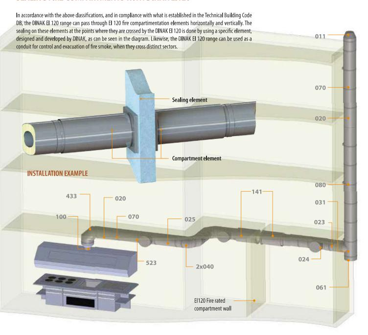
The DINAK EI120 range incorporates a stainless steel perimeter ring on the inside of the female end of the outer wall, on to which neutral, high temperature resistant, silicon sealant can be applied, and which guarantees perfectly airtight joints
